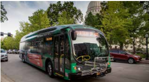
This all-electric bus has a battery range of up to 250 miles.
